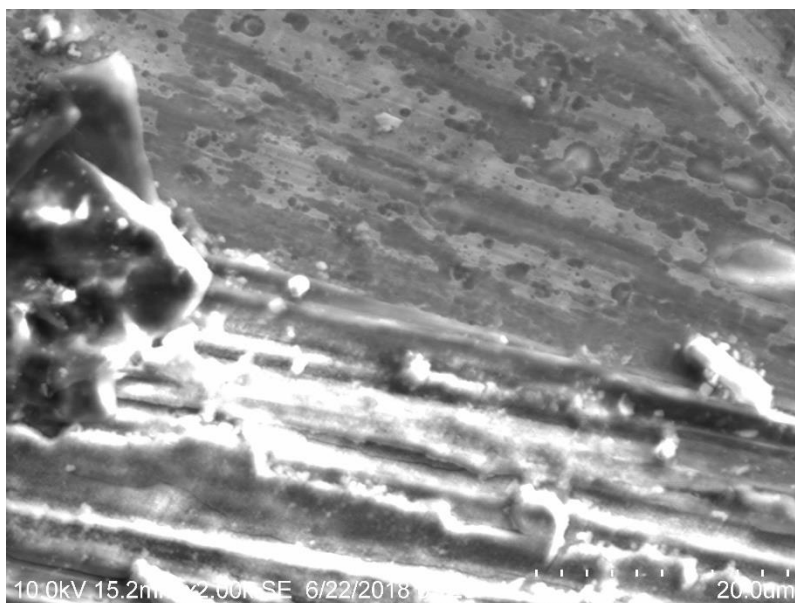
Figure 2 Secondary electron image of surface of nickel hydroxide exposed specimen.
